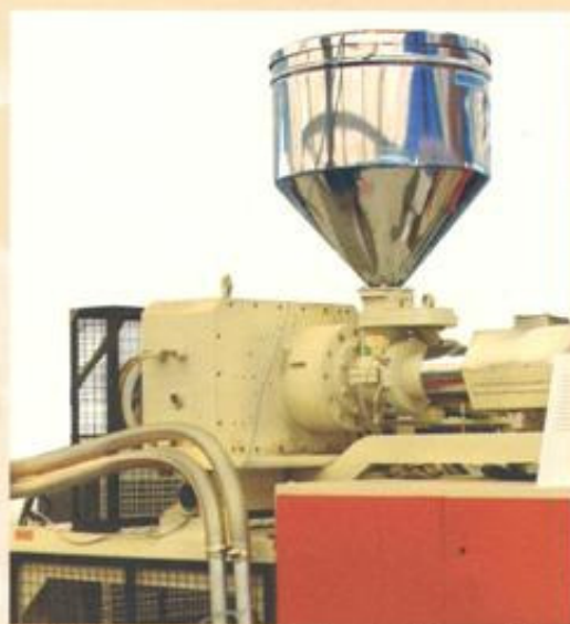
INGECO Gearbox fitted in Blow Molding machine
