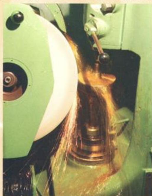
All Gears being Profile Ground on Imported Csepel Multi Flank Gear Grinder upto DIN Class 6/8
