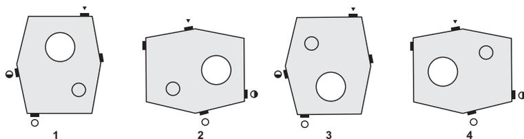
Units are fitted with Filler and Drain Plugs generally in the position shown
